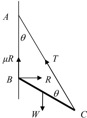
$$\begin{aligned}T \sin \theta(2p) &= W \sin 2\theta(p) \\T \sin \theta(2p) &= W 2 \sin \theta \cos \theta(p) \\T &= W \cos \theta\end{aligned}$$
