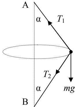
$$T_1 \sin \alpha + T_2 \sin \alpha = m(\ell \sin \alpha) \omega^2$$
